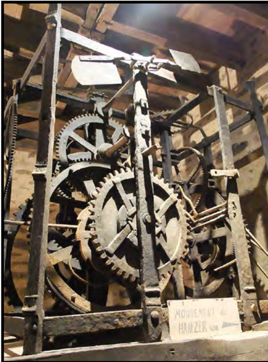
The Hamzer clock mechanism in Dinan, France, from 1498.
